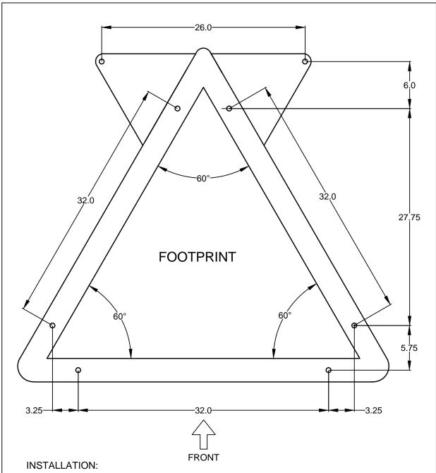
Use 8 each, ½" diameter Steel Bolts to secure the base as indicated, to a level floor and orientate the base so that the air/water separator and the foot switch is toward the front to allow full operator access.
